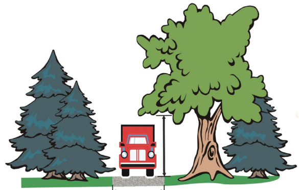
Fire trucks need clearance from surrounding vegetation
